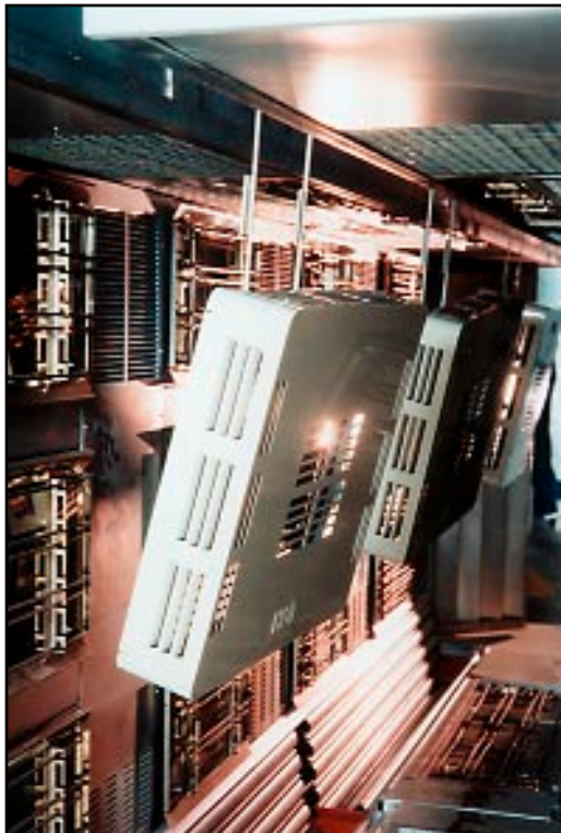
Photo 4-3: Curing powder coating in infrared oven. (Note: Red lighting is used to illustrate reflective surfaces.) Photograph by R. A. Flynn
