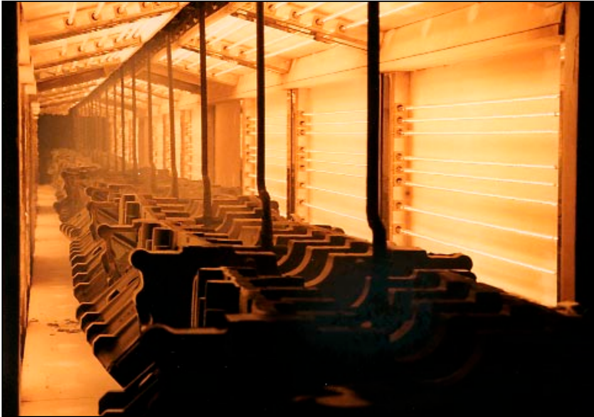
Photo 4-1: Powder coated engine blocks being cured by the ICS short wave infrared oven. Photograph courtesy of BGK Finishing Systems
