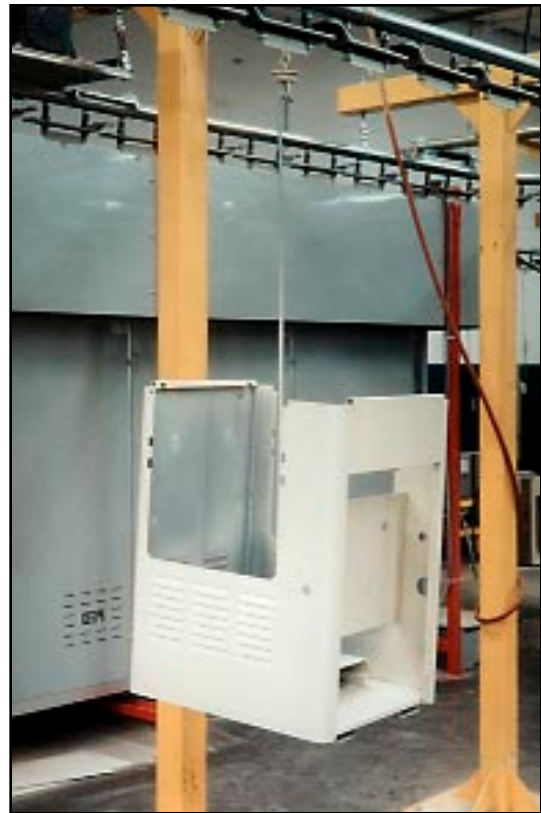
Photo 4-4: Cabinet body after powder spraying and curing. Infrared oven in background.
