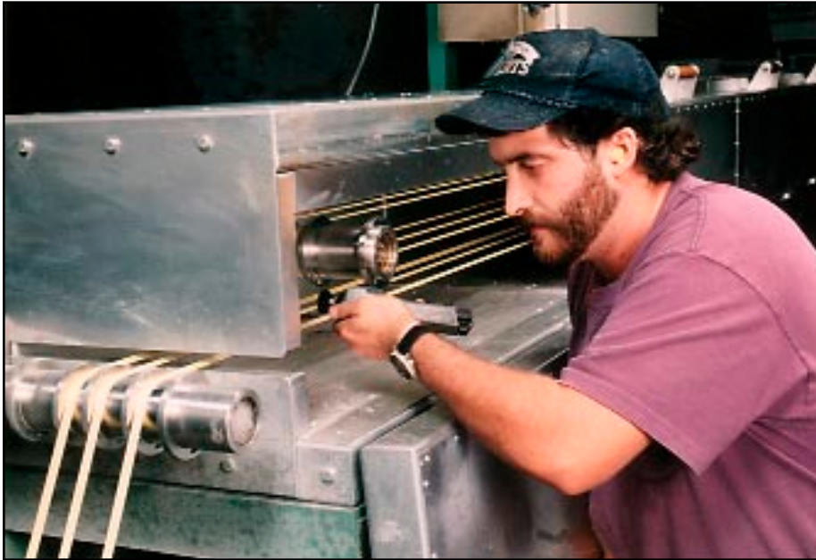
Photo 4-2: As a normal part of Dynaric's quality control, technician Karl Schmitt checks the roll speed of straps on the production line in the exit section of an IR oven. The side door has been opened for this test. The three-pass path of the strapping can be seen. Heat and roll speed must be properly maintained throughout the process to meet Dynaric's high standards of consistency.
