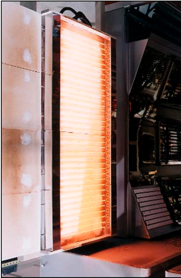
Photo 2-6: Short-Wave Infrared Booster Oven Section
