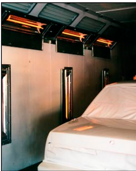
Photo 4-6: A Paint Job Curing
