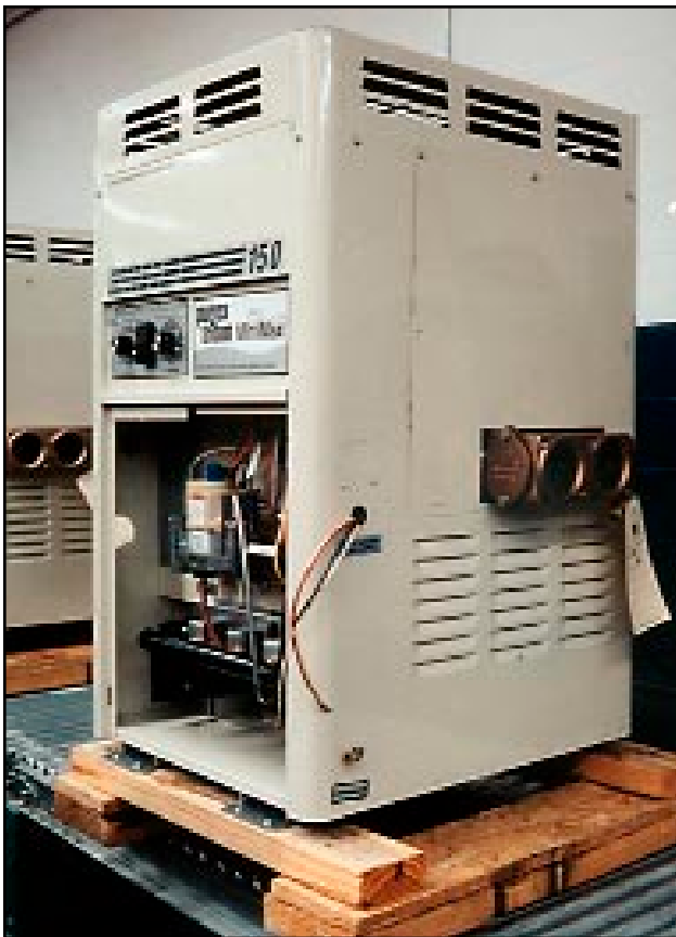
Photo 4-5: Assembled swimming pool heater awaiting final testing.
